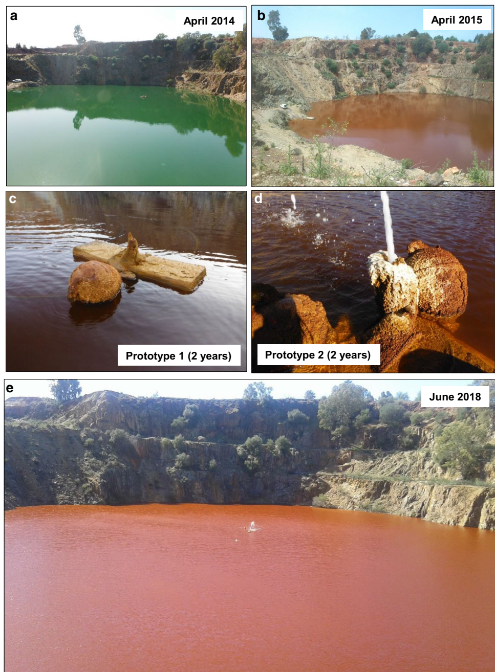
Fig. 9 Sequence of pictures showing the effects of the continuous pumping of gas-charged deep water to the pit lake surface: a aspect of the pit lake in April 2014, before the start of degassing; b aspect of the pit lake in April 2015, after 6 months of deep water pumping by two pilot-scale pipes; c, d aspect of the degassing pipes (Prototypes 1 and 2) after 2 years of operation (note massive formation of mineral coatings on the tap, foam platform and buoys); e panoramic view of the pit lake in June 2018 (note deep red colour resulting from high contents of dissolved Fe[III])
