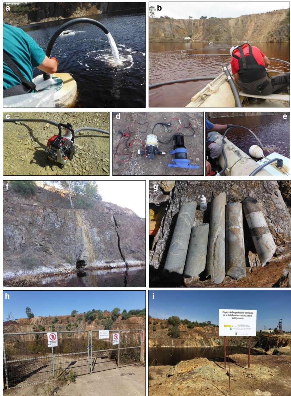
Fig. 3 Field pictures taken in the Guadiana acidic pit lake during the period 2017–2018: a activation of degassing Pipe 1; b installation of degassing Pipe 2; c Conventional high-speed motor pump initially used for pumping of degassing Pipe 2, which proved to be inefficient to pump the gas-charged deep water; d, e membrane pumps finally used to evacuate the gas-charged water from within the hoses and put degassing pipes 1 and 2 into operation; f detail of mine tunnel and big fracture in the pit walls at the northern part of the open pit; g remnants of drill cores found in the pit with abundant carbonate (calcite, dolomite) present in fractures and voids of the volcanic rocks; h, i warning signboards installed in the pit fence after the activation of Pipe 1
